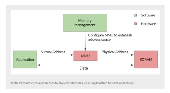
Each application's virtual address space is unique. When an application accesses a valid address within its own space, the MMU translates that virtual address into the corresponding physical location in memory. The MMU generates a page fault if an application attempts to access a memory address outside its defined space. This traps into the kernel, which then terminates the offending application, ensuring that the unauthorized access does not complete. For example:
