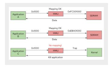
Applications A and B have overlapping virtual addresses (e.g., 0x1000) but are mapped to different physical memory locations by the MMU.
